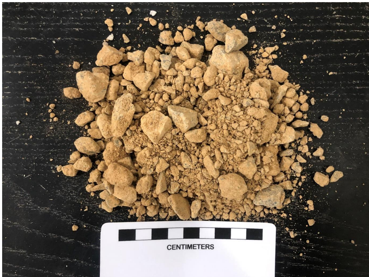
Plate 1: Photograph of the sample as provided, showing the poorly sorted, angular roadbase particles coated in abundant, light orangish-brown fines.
