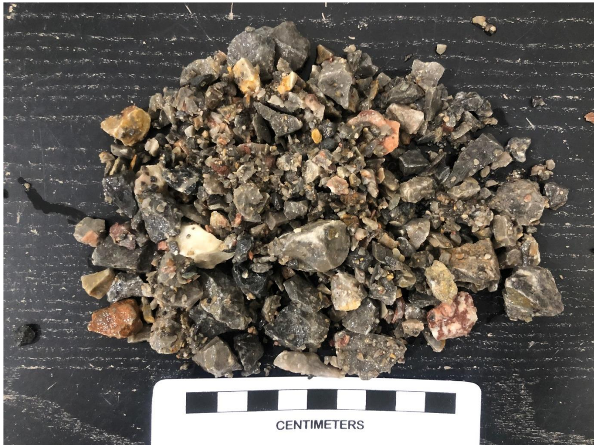
Plate 2: Photograph of sample when wetted, which removes the goethitic fines leaving the variably coloured limestone particles.
