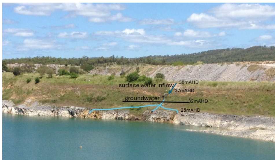
Figure 32 The Seep and groundwater seepage into Pit 3 – 4 March 2015
