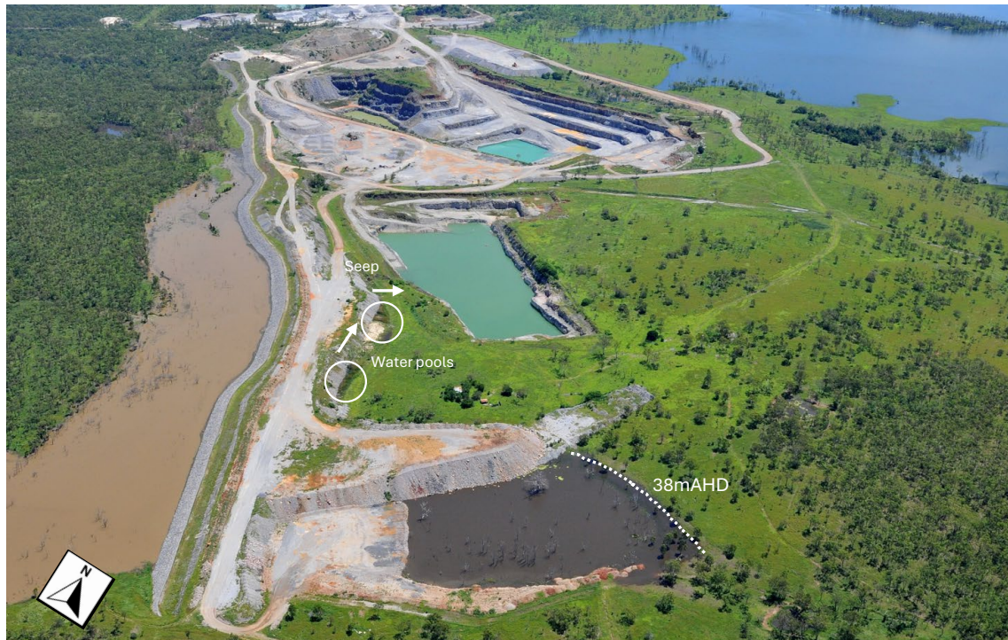
Figure 34 Western bund wall surface water flow into Pit 3 on 22 February 2015
