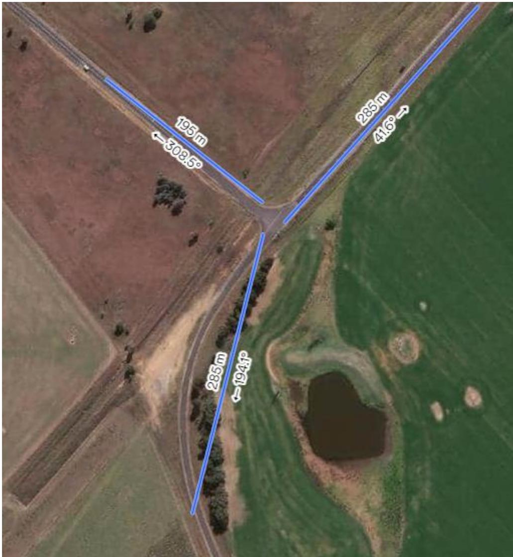
Sight distance from the southern approach is restricted. However, mitigation measures have been installed on the western Cunningar Road approach in the form of raised rumble bars and signage as shown in Figure 10.
