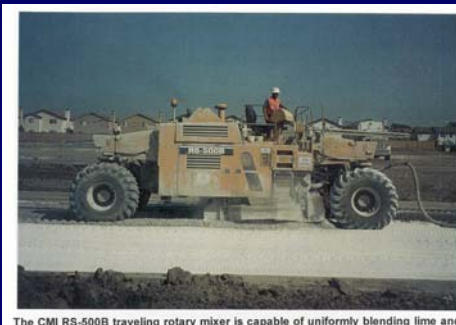
The CMI RS-500B traveling rotary mixer is capable of uniformly blending lime and soil to a depth of 20 inches. The mixer is designed specifically for soil stabilization and asphalt pulverization. The CMI RS-500B is equipped with an on-board computer that controls the mixing depth and flow of water through the pump system.
