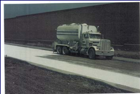
Standard rubber-tire spreader equipped with an auger system and vane feeder for controlled dry product distribution.
