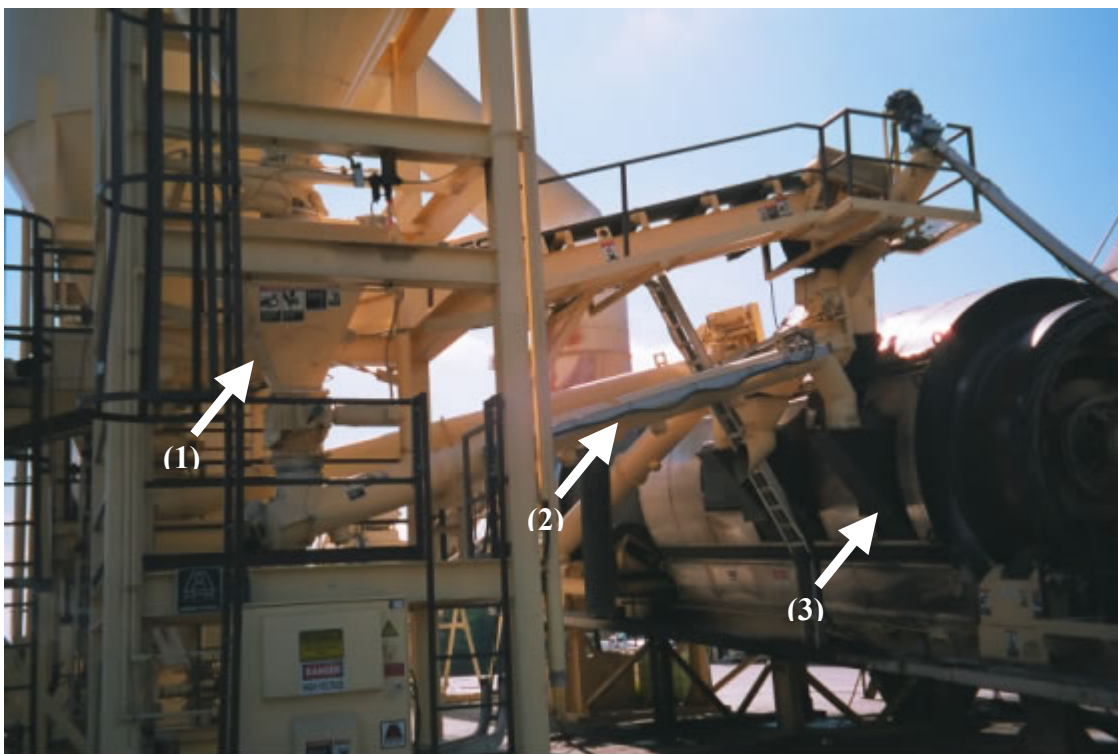
Figure 2: Weigh pot (1) dispenses hydrated lime through rotary vane feeder that feeds hydrated lime into a screw conveyor (2) and is then injected into outer shell of double drum (3).
